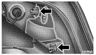
3. Grasp the taillight and pull firmly outward pushing gently on the studs from inside to disengage the light housing.
